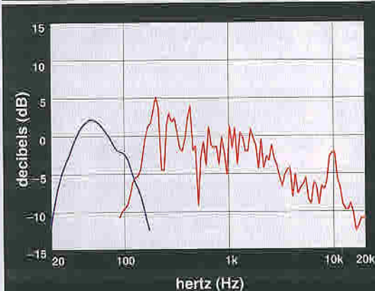
L/R/Center/Surround 150 Hz to 10.3 kHz \pm 7.3 dB Subwoofer 29 Hz to 106 kHz \pm 2.5 dB
